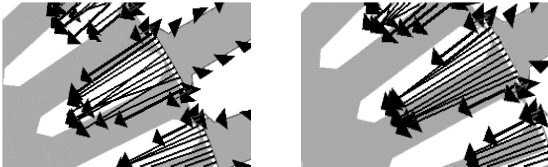
Figure 2 - Local force distribution on a tooth. (a) Rotor bar in front of a tooth. (b) Rotor bar dislocated of 10 degrees in relation to the tooth.
